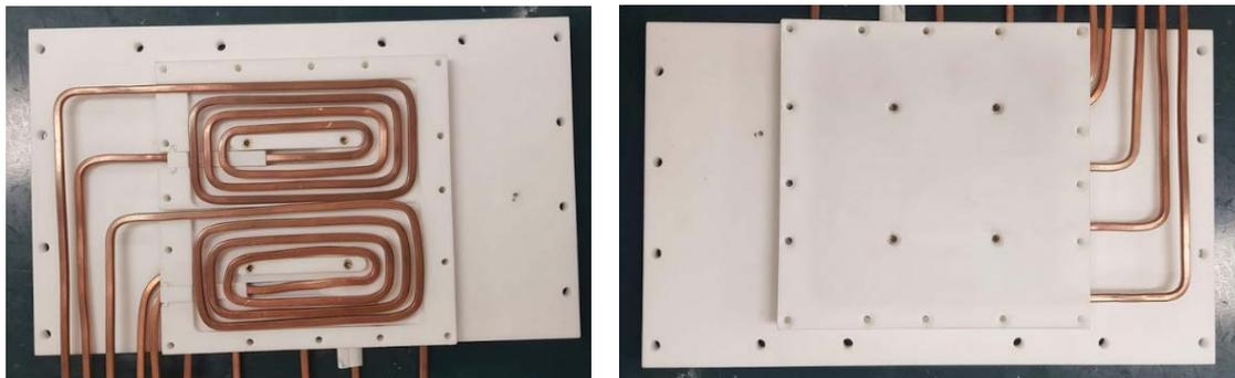
**Figure 11:** Gradient polyamide structure. Y-coil layer (left). Final assembly (right).
