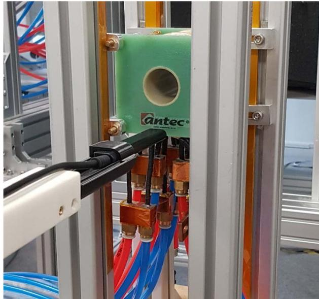
**Figure 8:** Picture of the Prepolarizer magnet during the experimental characterization at MRILab (i3M).
